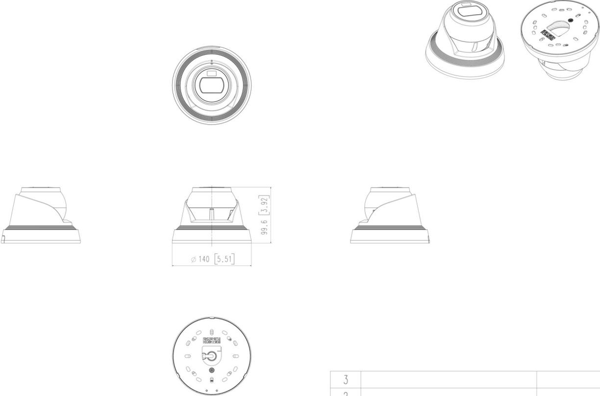
Technical CAD drawings of the QNE-C8013RL camera. The drawings include:
