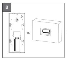
Stick the device onto mounting box of door phone or wall. The installation is done.
