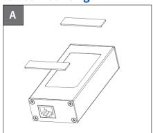
Stick two double-sided tapes on the back of device.
