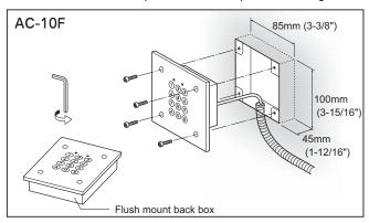
When this unit is to be used with the JF-DV, please refer to the illustration below when installing it. Please also refer to "TEMPLATE FOR AC-10S MOUNTING BRACKET(SCALE 1:1)"(page 42).
