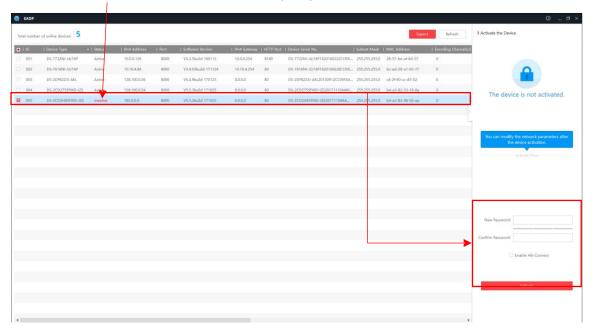
V. Once the device is Active you will be able to Modify Network Parameters (use ping test to find an available IP OR use the IP range your client has specified)
