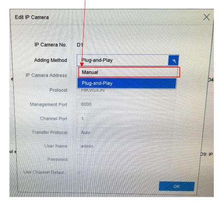
vi) Enter the IP Address that you have assigned to the camera earlier and enter the password you used to activate the camera and click OK
