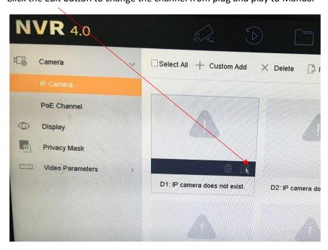
Change the Adding Method to manual by clicking the drop-down box (NOTE: Once a network camera has been assigned this channel cannot be used for plug & play, for example cannot plug camera into this PoE Port)
