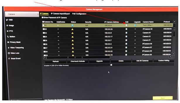
Change the Adding Method to manual by clicking the drop-down box (NOTE: Once a network camera has been assigned this channel cannot be used for plug & play, for example cannot plug camera into this PoE Port)
