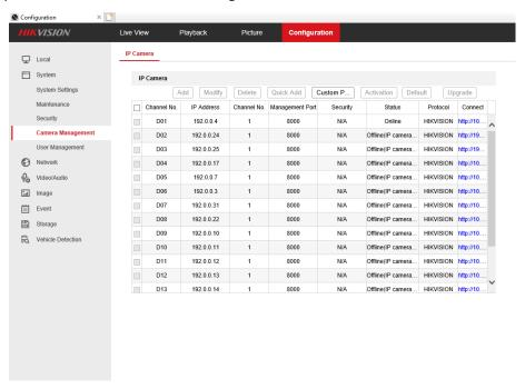
Select the camera channel that you wish to modify (NOTE: Once a network camera has been assigned this
