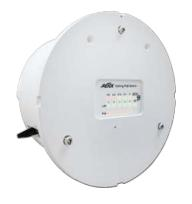
AETEK's managed C62-050-030 Ceiling PoE Switch line with one PoE PD input port, five PoE PSE outport ports, and visible LED indicator benefits from low-cost installation quick diagnostic, and low-voltage safety DC power deployment. C62-050-30-B unparalleled daisy-chain PoE feature extends long range PoE up to 300m over cat 5e/cat 6 cable without extra AC/DC power adapter in ceiling. Furthermore C62-050-30-B provides DC 12V & DC 24V output for DC device.
