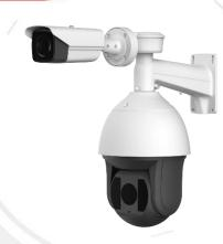
Hikvision DS-2TX3636-25A Thermal Smart Linkage Tracking Systems is formed by one fixed camera and one PTZ camera. The PTZ camera smartly tracks multiple moving targets, and the fixed camera offers the panoramic view. The linkage of both can be realized by the client software.
