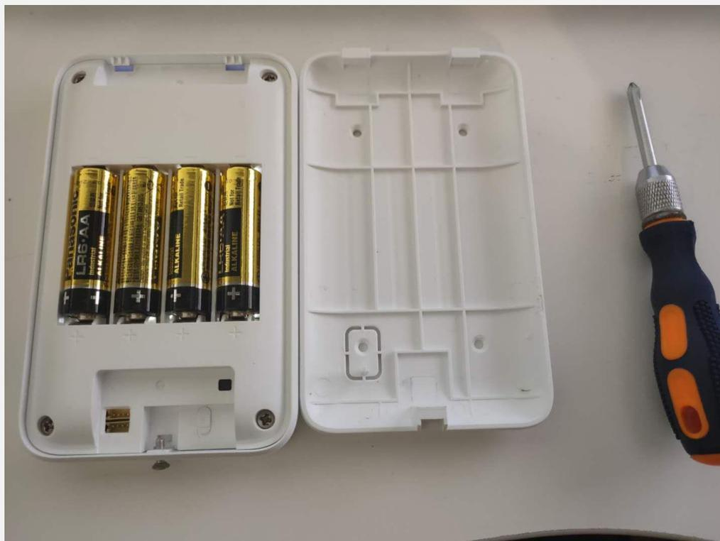
Open the keypad with screwdriver
