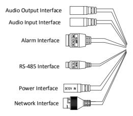
Figure 2-3 Cables of Thermal Turret Camera
