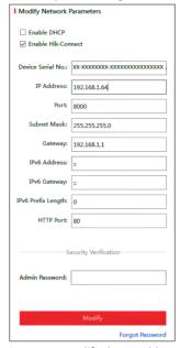
Figure 4-4 Modify the IP Address
