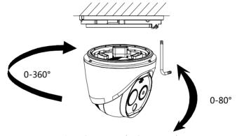
Figure 3-7 Mount the Camera Body
