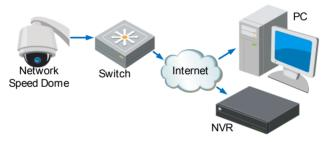
Figure 4-1 Wiring over LAN
