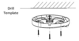
Figure 3-6 Mount the Camera Base
