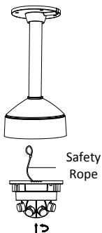
Figure 2-17 Install the Camera to the Bracket (1)
