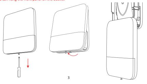
3.Attach the sounder to the required place with the top screw. Make the sounder horizontal by resorting to the gradienter.
