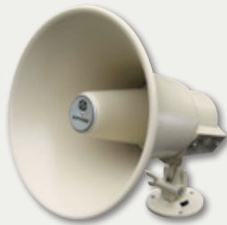
AH-32TN Horn Speaker • 25/70V, 32W • Indoor or outdoor use • Surface mount Bell Diameter: 8-1/8" Depth: 9"
