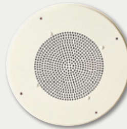
SP-2570N Ceiling Speaker • 8Ω, 25/70V, 5W • Indoor use • Flush mount Diameter: 12-7/8" Baffle Diameter: 8"
