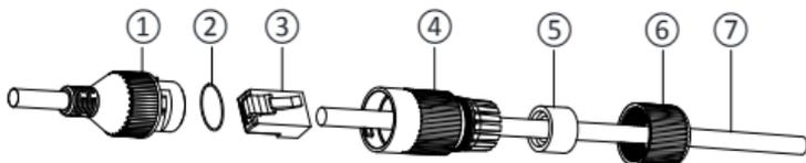
Figure 2-10 Waterproof Accessory Components
