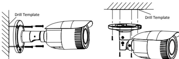
Figure 2-6 Secure the Camera
