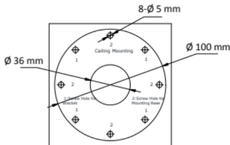
Figure 2-5 Drilling Holes in the Wall/Ceiling
