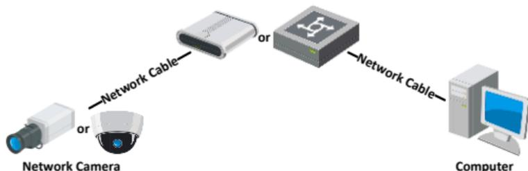
Figure 3-2 Connect via a Switch or a Router
