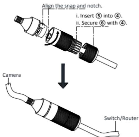
Figure 2-11 Waterproof Accessory Installation
