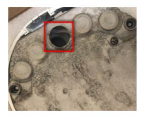
f. Pay attention when closing the lid as some o the domes have a standoff on the lid that has to go into a cavity on the base.
