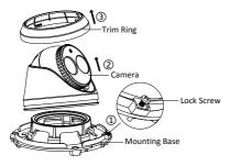
Figure 2-1 Disassemble the Camera
