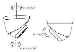
Figure 2-35 Adjust the Lens
