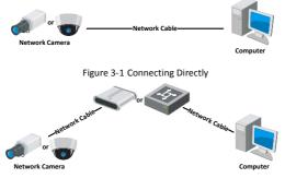
Figure 3-2 Connecting via a Switch or a Router
