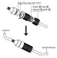
Figure 2-44 Waterproof Accessory Installation
