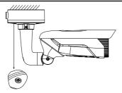
Figure 2-4 Tighten the Lock Screw
