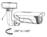
Figure 2-9 Adjust Pan Angle
