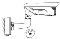
Figure 2-8 Tighten the Lock Screw
