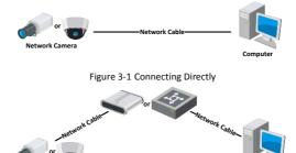
Figure 3-2 Connecting via a Switch or a Router
