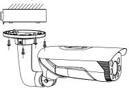
Figure 2-3 Install Camera
