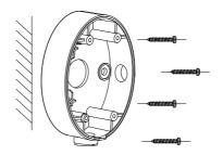
Figure 2-6 Install Junction Box
