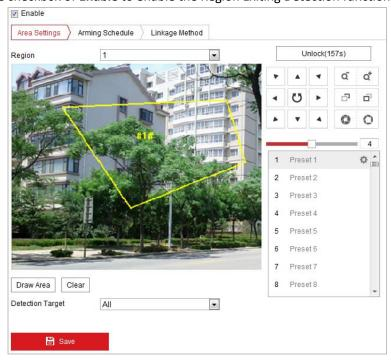
Figure 5-26 Configuring Region Exiting Detection
