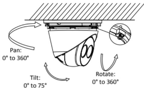
Figure 2-28 Adjust Surveillance Angle
