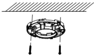
Figure 2-19 Install the Mounting Base
