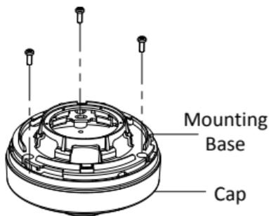
Figure 2-40 Fix Mounting Base
