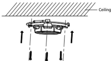
Figure 2-4 Secure the Mounting to the Ceiling
