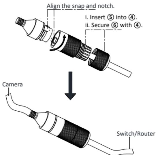
Figure 2-44 Waterproof Accessory Installation
