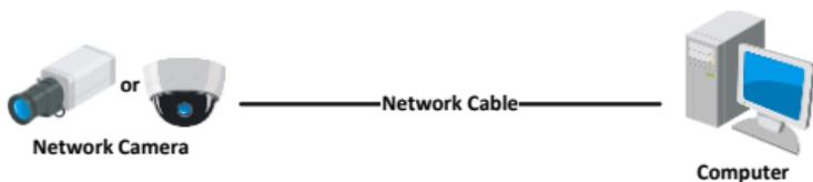
Figure 3-1 Connecting Directly
