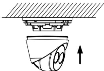
Figure 2-27 Install the Camera
