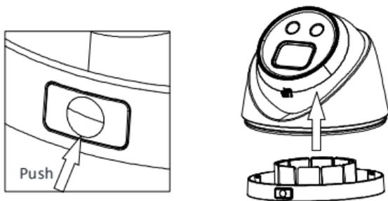
Figure 2-30 Remove the Bottom Base
