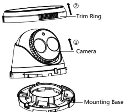
Figure 2-9 Disassemble the Camera
