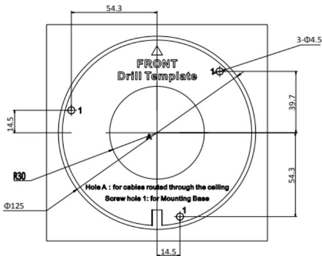
Figure 2-32 The Drill Template
