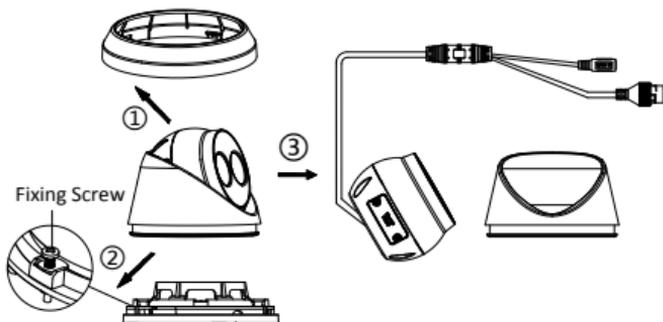
Figure 2-23 Disassemble the Camera
