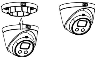
Figure 2-34 Secure the Camera to the Mounting Base
