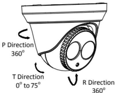
Figure 2-7 Adjust the Lens
