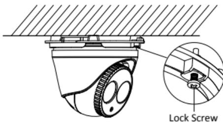
Figure 2-6 Loosen Lock Screw
