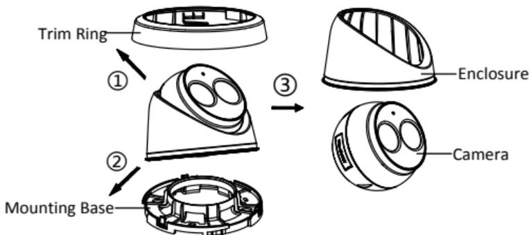
Figure 2-15 Disassemble the Camera
