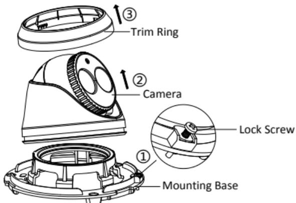
Figure 2-1 Disassemble the Camera
