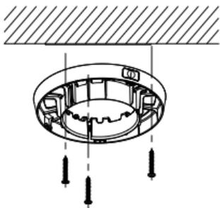
Figure 2-33 Secure the Mounting to the Ceiling
