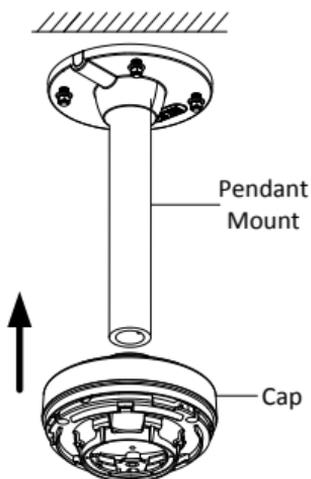
Figure 2-41 Install the Cap
