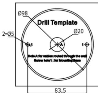
Figure 2-10 The Drill Template
