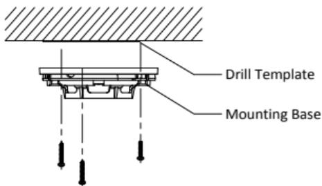
Figure 2-26 Fix Mounting Base
