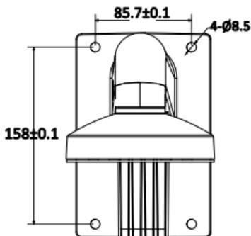
Figure 2-36 Dimension of Demonstrated Wall Mounting Bracket
