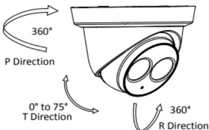
Figure 2-21 Adjust the Lens
