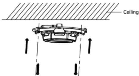
Figure 2-12 Secure the Camera to the Ceiling
