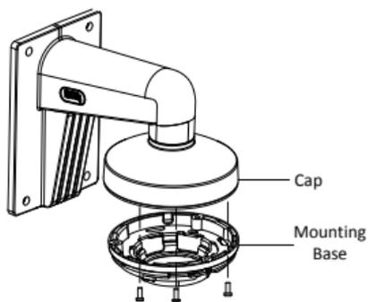
Figure 2-37 Fix Mounting Base
