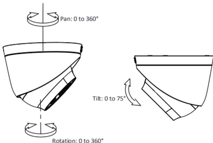
Figure 2-35 Adjust the Lens
