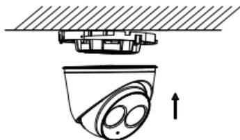
Figure 2-20 Install the Camera
