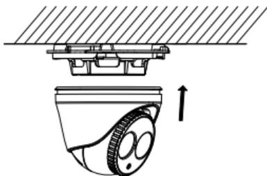
Figure 2-5 Secure the Camera to the Mounting Base
