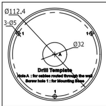
Figure 2-2 The Drill Template
