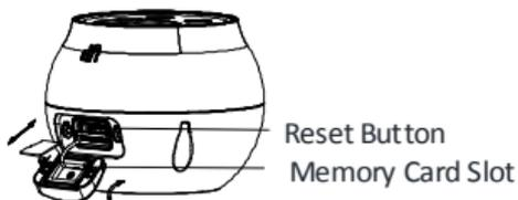
Figure 2-31 Insert the Memory Card into the Slot
