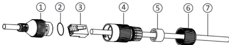
Figure 2-43 Waterproof Accessory Components
