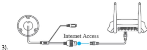
Figure 5-3 Connect a Router
