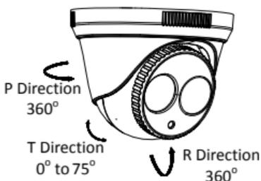
Figure 2-13 Adjust the Lens
