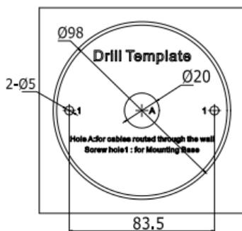
Figure 2-18 The Drill Template
