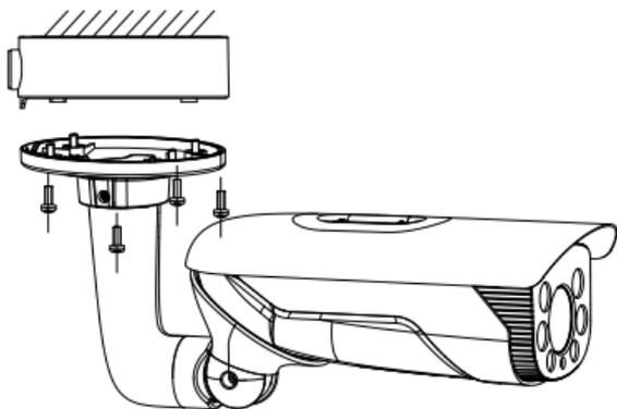
Figure 2-3 Install Camera
