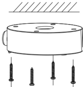
Figure 2-2 Install Junction Box
