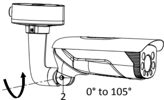
Figure 2-10 Adjust Tilt Angle
