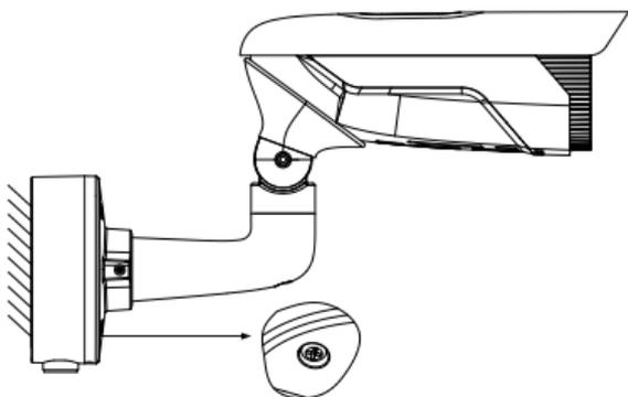
Figure 2-8 Tighten the Lock Screw
