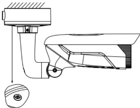
Figure 2-4 Tighten the Lock Screw
