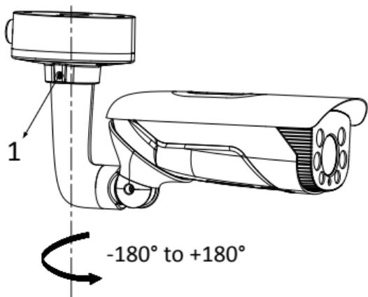
Figure 2-9 Adjust Pan Angle
