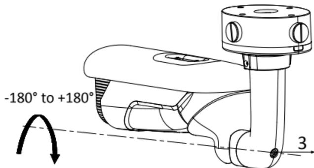
Figure 2-11 Adjust the Rotation Angle
