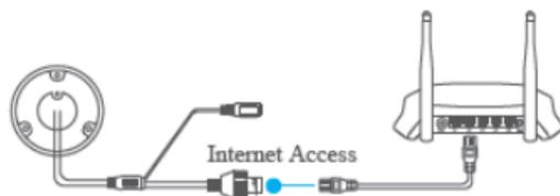
Figure 5-3 Connect a Router
