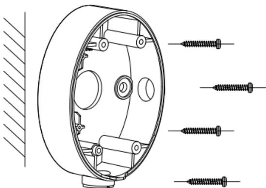
Figure 2-6 Install Junction Box
