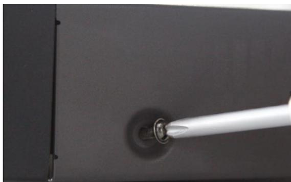
2. Install the HDD using the provided screws and fasten the screws on the bottom to fix the HDD.
