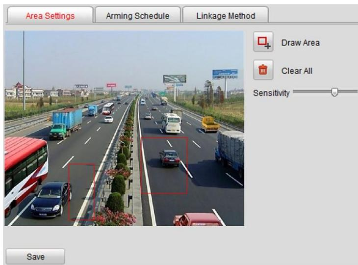
Figure 8.11 Motion Detection-Area Settings
