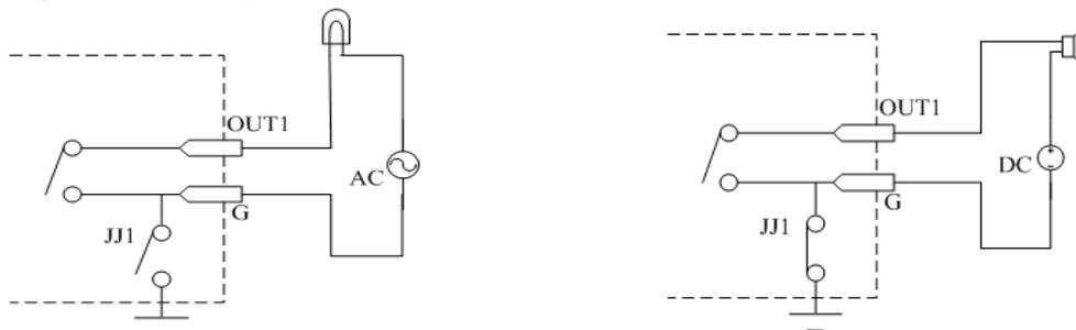
Figure 2.11 Alarm Output Connections
