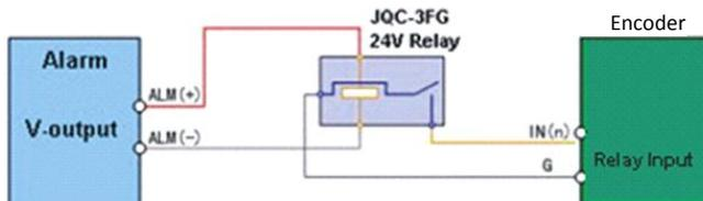
Figure 2.10 Alarm Input Connections for Normal Alarm
