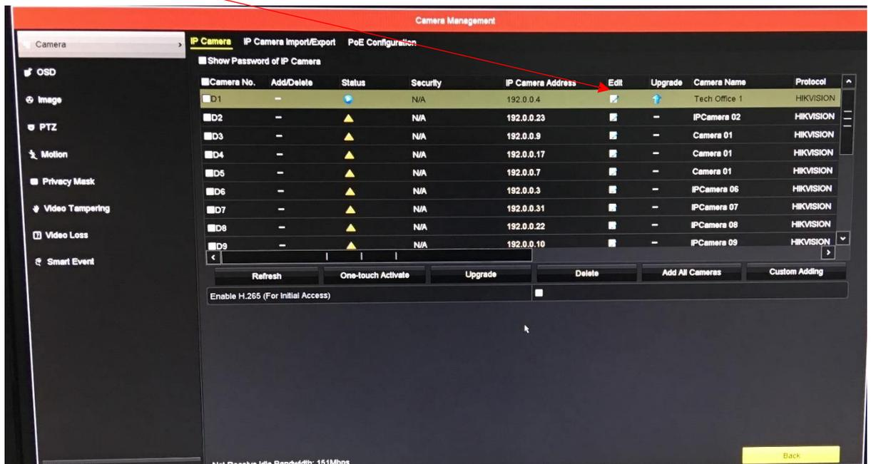
Change the Adding Method to manual by clicking the drop-down box (**NOTE: Once a network camera has been assigned this channel cannot be used for plug & play, for example cannot plug camera into this PoE Port**)
