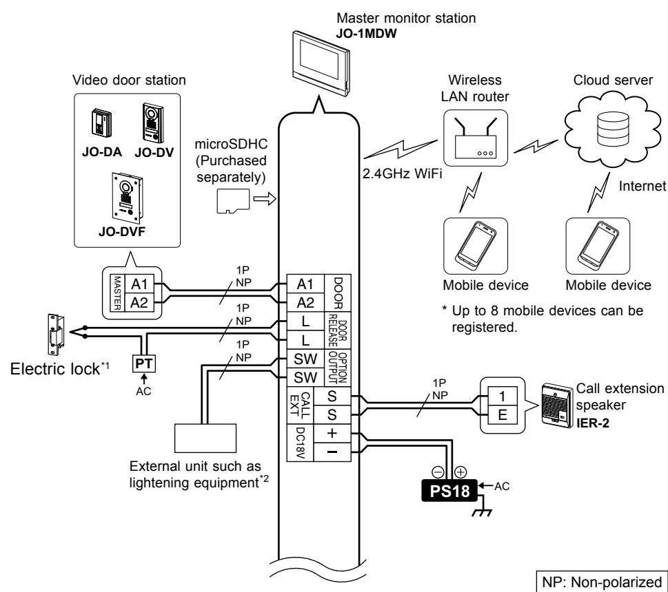
\*1: An EL-12S (AC 12 V, 0.125 A, DC 12 V, 0.2 A) or equivalent part and a separate AC transformer (or power supply) are required. Door release contact: AC/DC 24 V, 1 A (Minimum contact: 100 mV DC, 0.1 mA) (N/O dry closure contact L, L).
