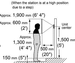
(When the station is at a high position due to a step)
