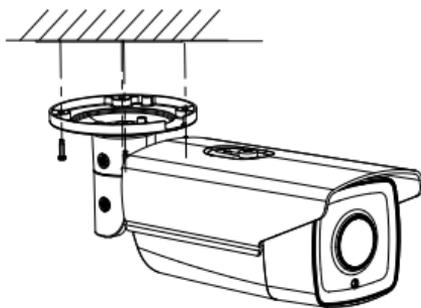
Figure 2-4 Install the Camera
