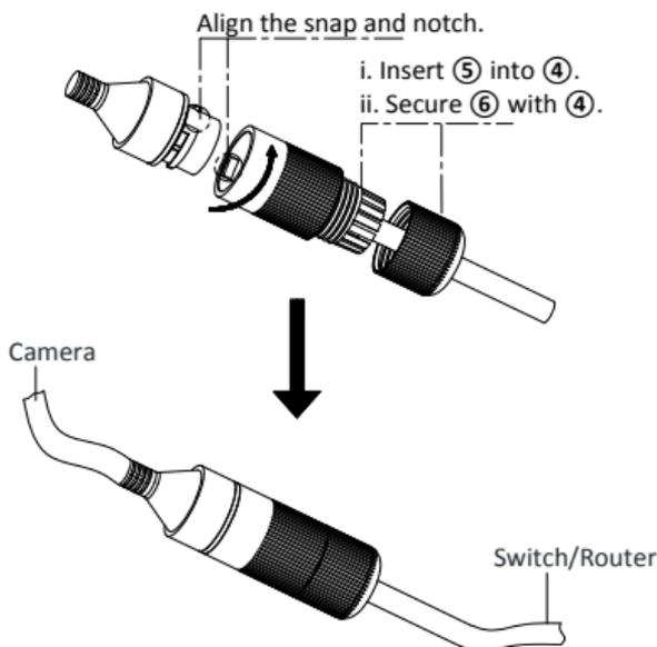
Figure 2-11 Water-proof Accessory Installation
