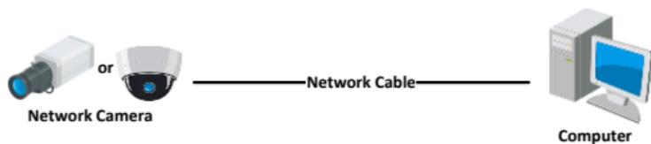
Figure 3-1 Connecting Directly
