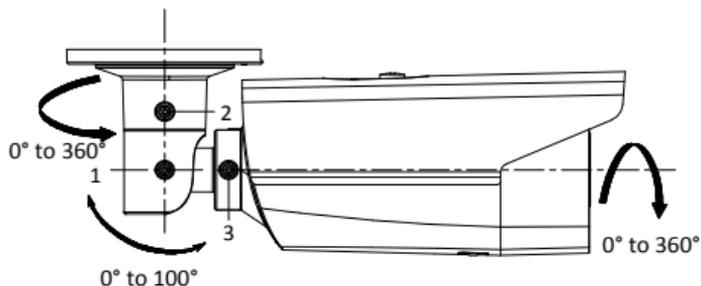
Figure 2-5 Adjust the Surveillance Angle
