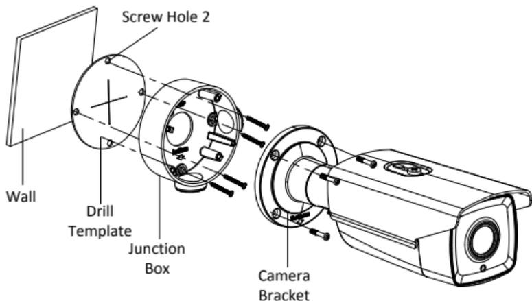
Figure 2-8 Installation with a Junction Box
