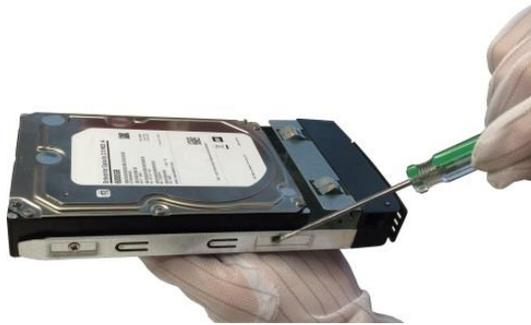
Figure 2. 9 Fix the Hard Disk
