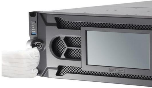
Figure 2. 12 Reinstall the Cover and Lock the Panel
