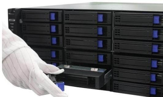
Figure 2. 8 Pull out Slot
