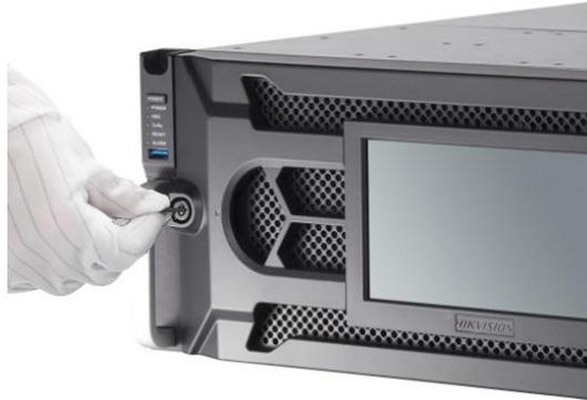
Figure 2. 6 Unlock the Panel
