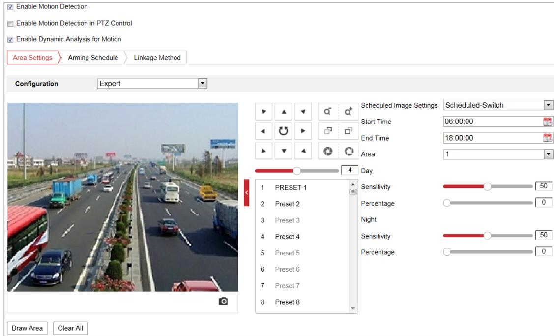
Figure 5-10 Motion Detection Settings-Expert
