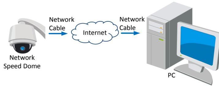
Figure 2-11 Accessing the Camera with Static IP Directly
